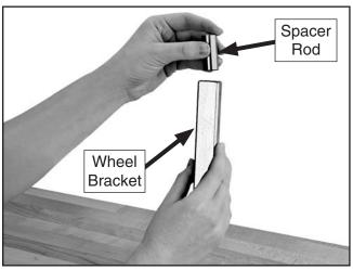
**Figure 4.** Inserting spacer rod into wheel bracket.
